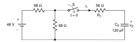
At time t = 0, switch S is closed and kept closed for the rest of the time.
