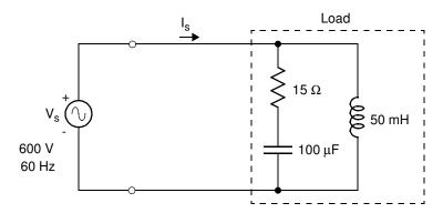
The rms value of the source  $V_s$  is 600 V. The phase of the source  $V_s$  is 0.
