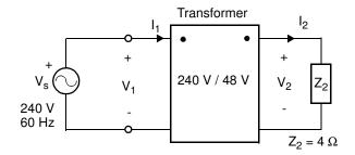
The transformer parameters are given:  $R_s = 3.6 \Omega$ ,  $X_s = 7.2 \Omega$ ,  $R_m = \infty$ ,  $X_m = \infty$ .
