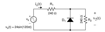
The conduction voltage of diode  $D_1$  is equal to  $V_F = 0.7$  V.
